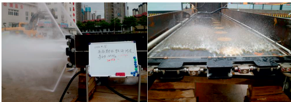
(b) high-pressure water jet (in testing)
