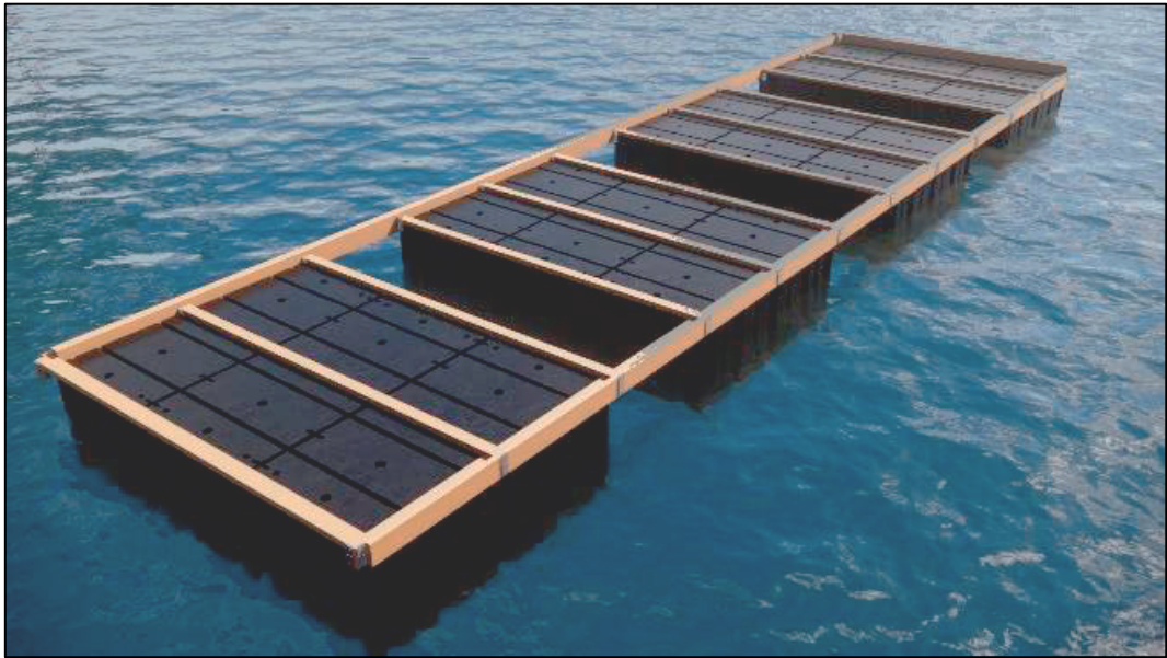
Figure 4: Rendering of a section of the floating foundation (Note: An outer wood-framed array before the decking and cabin structure have been installed)
