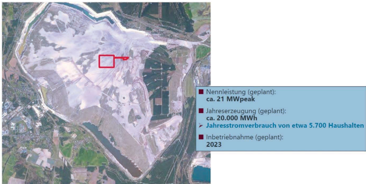
Fig. 1: location of the PV-system on the Cottbus Ostsee
